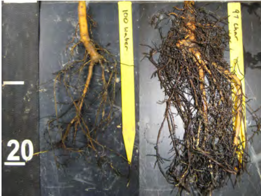
No Treatment (right) 5% biochar + compost top dressing Tree roots at 18 months in compacted soils. Photo: Morton Arboretum Soil Science Laboratory
